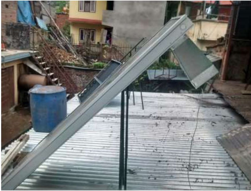
Figure 4.3 Test Setup with AC blower connected at the outlet of SAH
