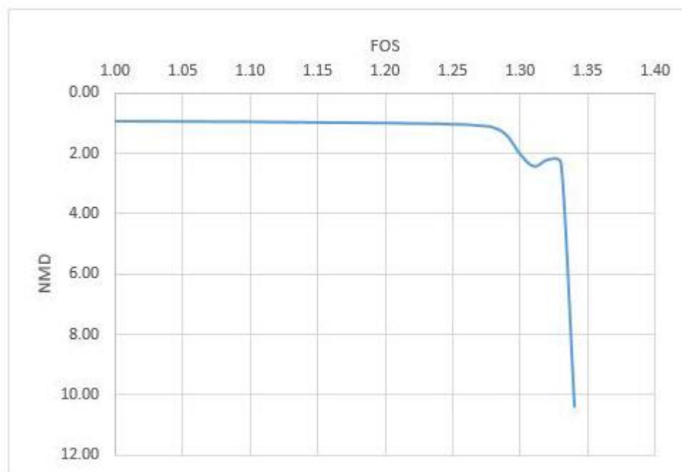
Figure 0.8 FOS plotted against Normalized Maximum Displacement (NMD) of general slope having \phi=35 degrees and X_p/X=1
