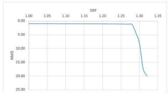
Figure B.5 FOS for general slope for without piles for \phi=35 degrees
