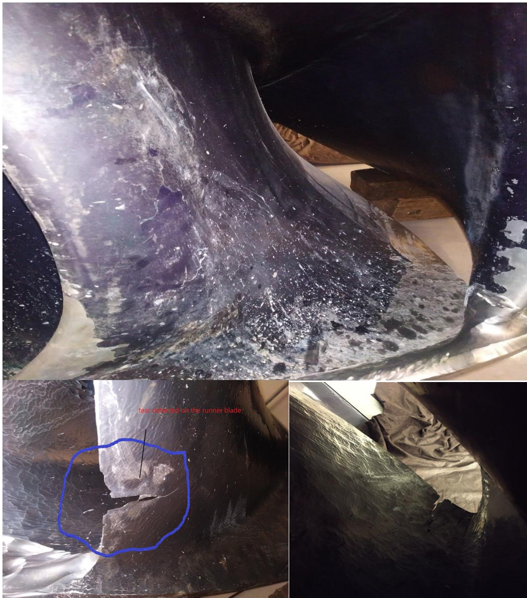
Figure 4. 16: Erosion pattern and tear in the trailing edge
