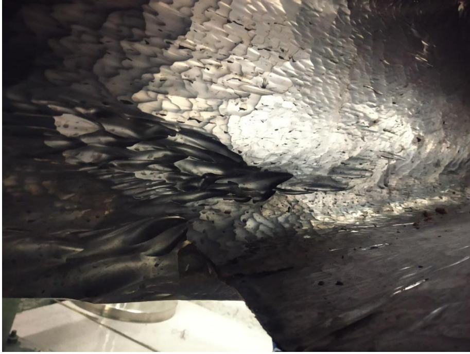
Figure A.5: Erosion detected in joining of shroud and blade (inlet side of Shroud)
