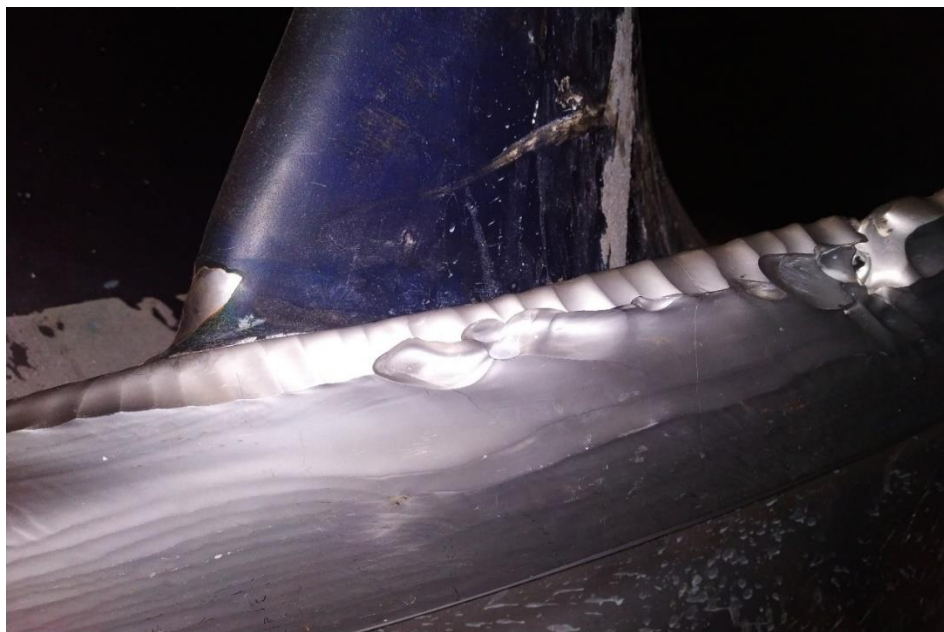
Figure A.4: Erosion detected in the leading edge and band side
