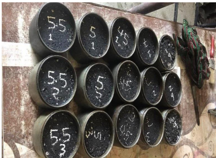
Figure 7 Prepared Asphalt specimens for 8% steel slag filler content
