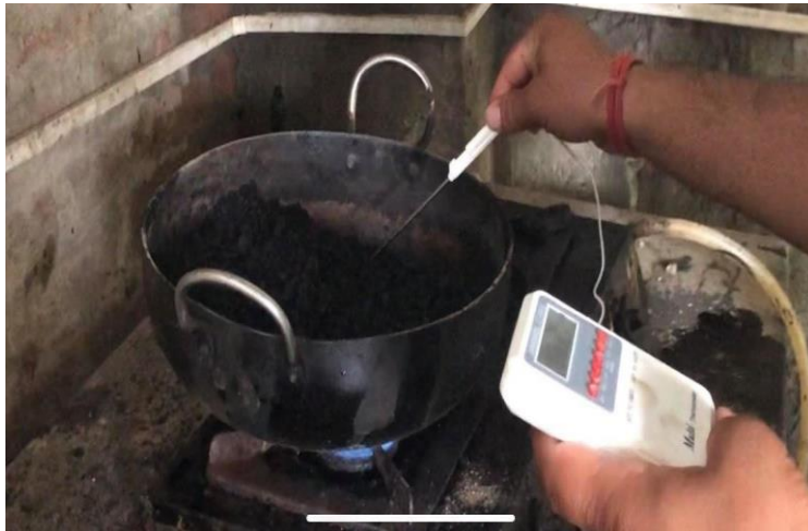
Figure 8 Measuring temperature of Asphalt mix
