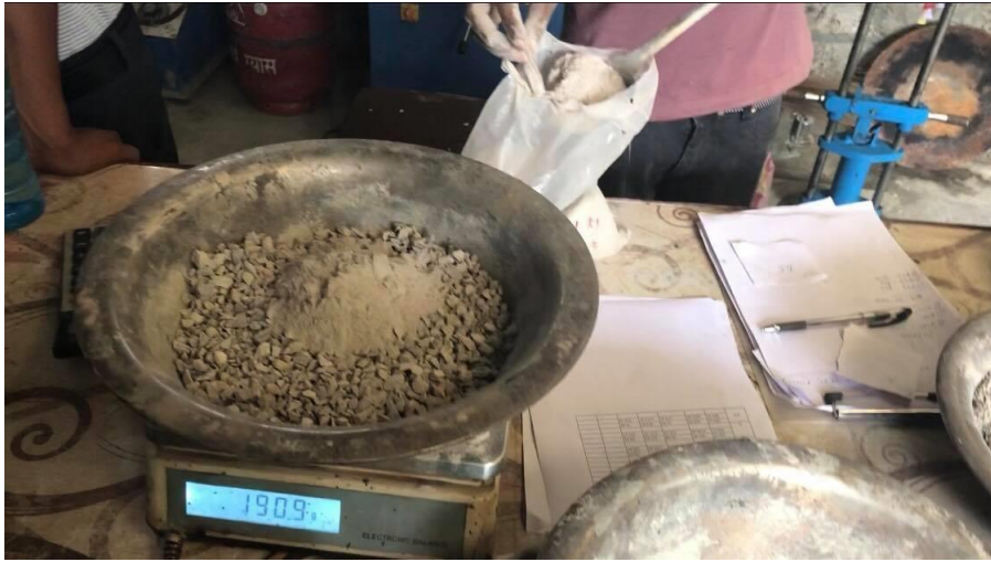
Figure 9 Mixing of steel slag on aggregate mix
