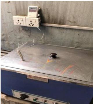
Figure 11 Samples at Hot water bath at 60 Degree Celcius for 30 min before Marshall Test
