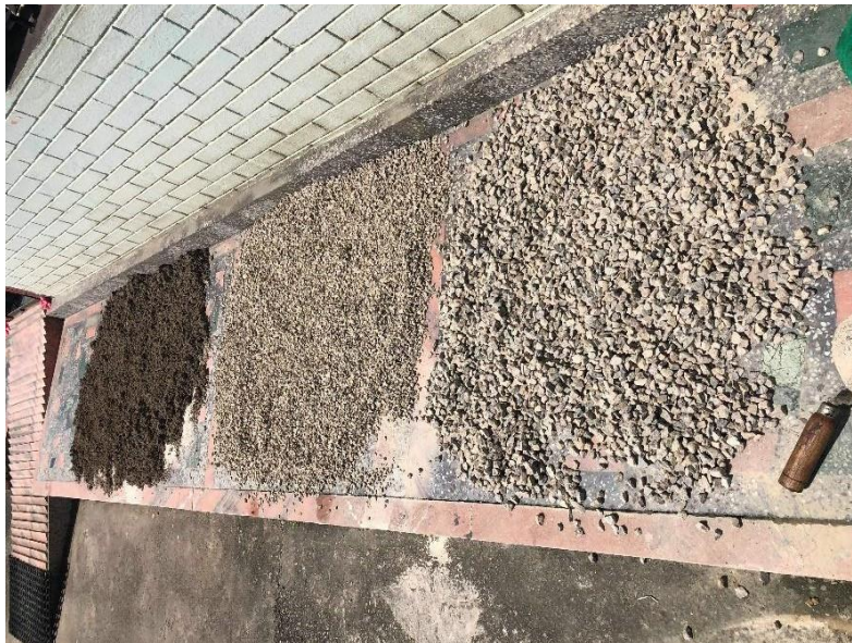
Figure 2 Aggregates used in Marshall Test
