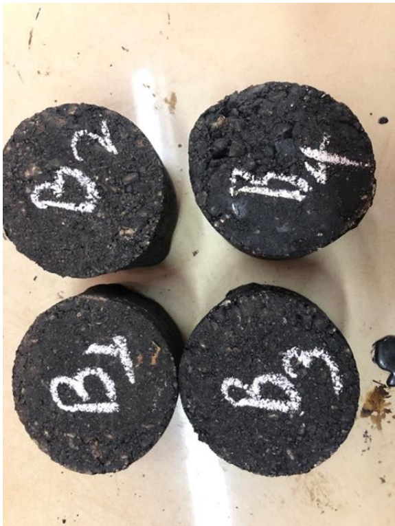
Figure 13 Marshall Sample for Retained Stability Test
