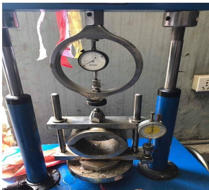
Figure 6 Marshall Stability test setup
