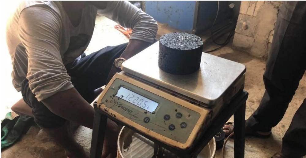
Figure 10 Weighing of specimen before Marshall test
