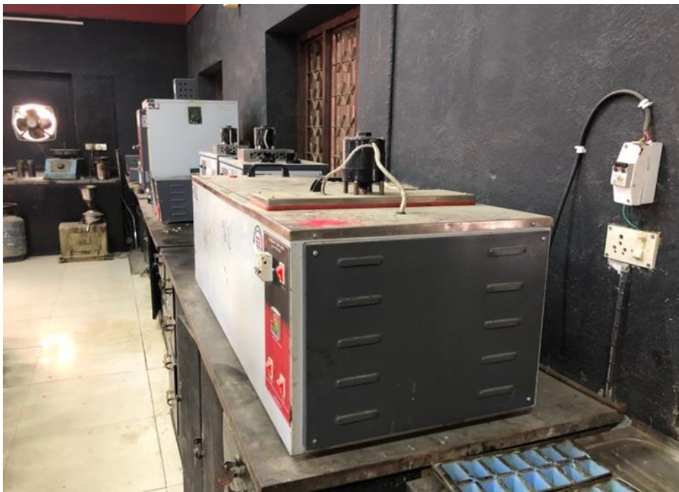
Figure 14 Water Bath for Retained Stability Test
