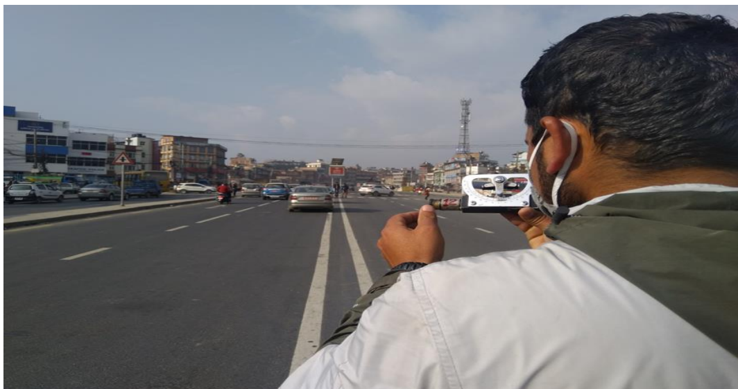
Figure 3.4 Geometric Data Collection Using Measuring 30m Tape, Abney Level and Prismatic Compass.
