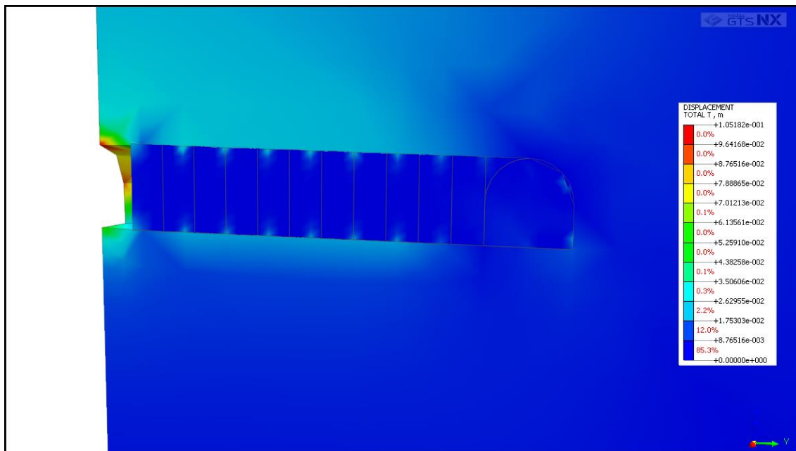
Figure 8-12: Displacement around Adit Connection, Stage 1
