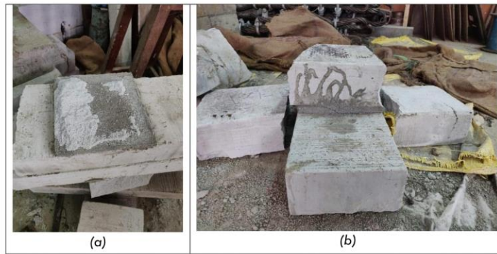
227 Figure 8 Different failure patterns of AAC cross-couplet specimen: (a) partial block-mortar 228 interface failure (Type-II), (b) complete tensile failure of block (Type IV)
