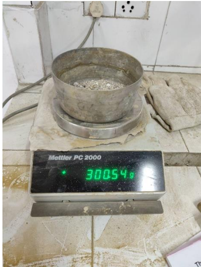
Figure 14 Weighing of Sieve Sample
