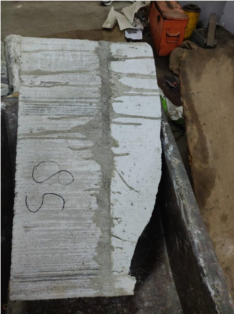
Figure 27 Failure of block (Type A)
