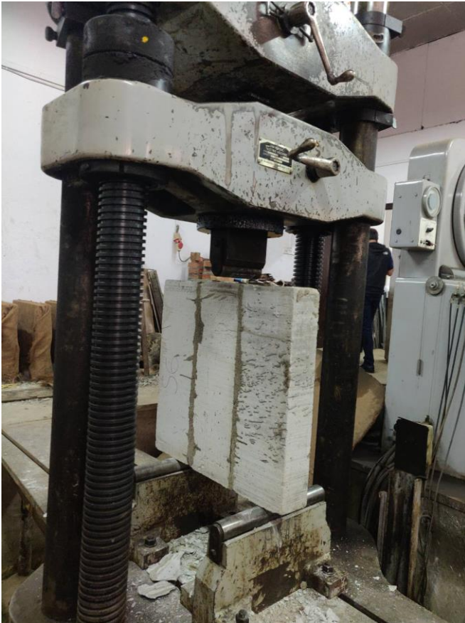
Figure 23 Shear Strength Test of Triplet Sample
