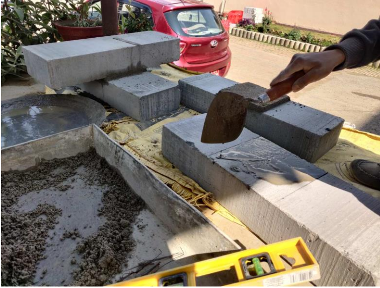
Figure 20 Preparation of Cross-Couplet Samples
