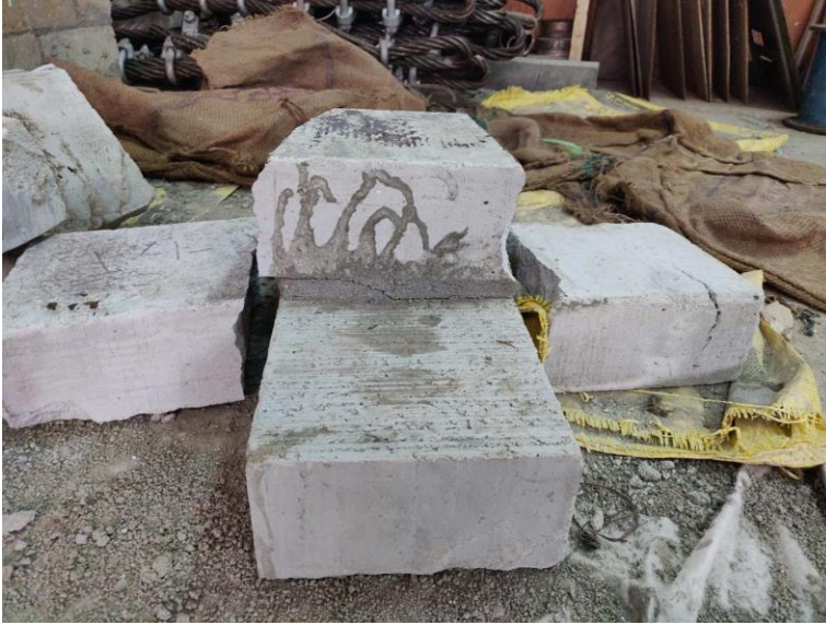
Figure 25 Complete Tensial Failure of Block (Type IV)
