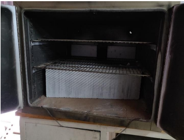
Figure 11 Drying of AAC Block
