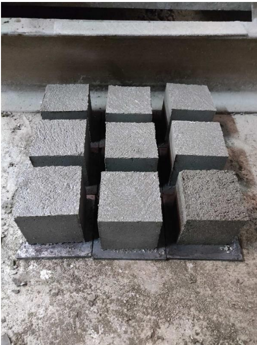
Figure 17 Mortar Cube Samples
