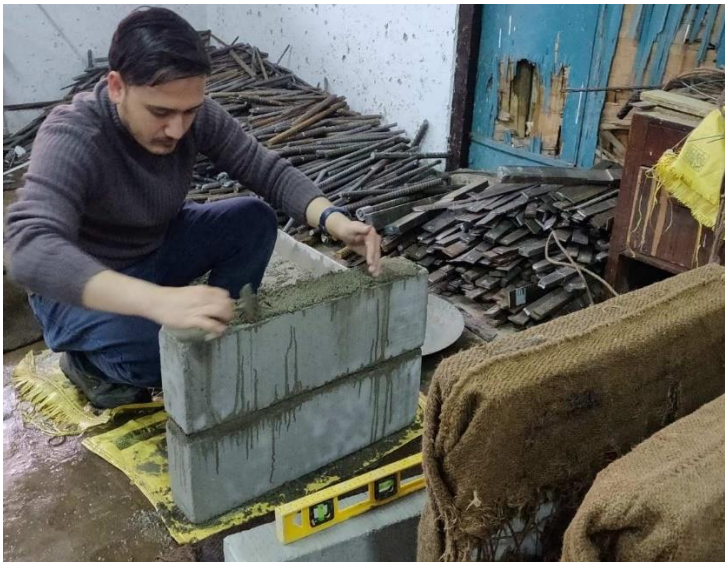
Figure 19 Preparation of Triplet Samples
