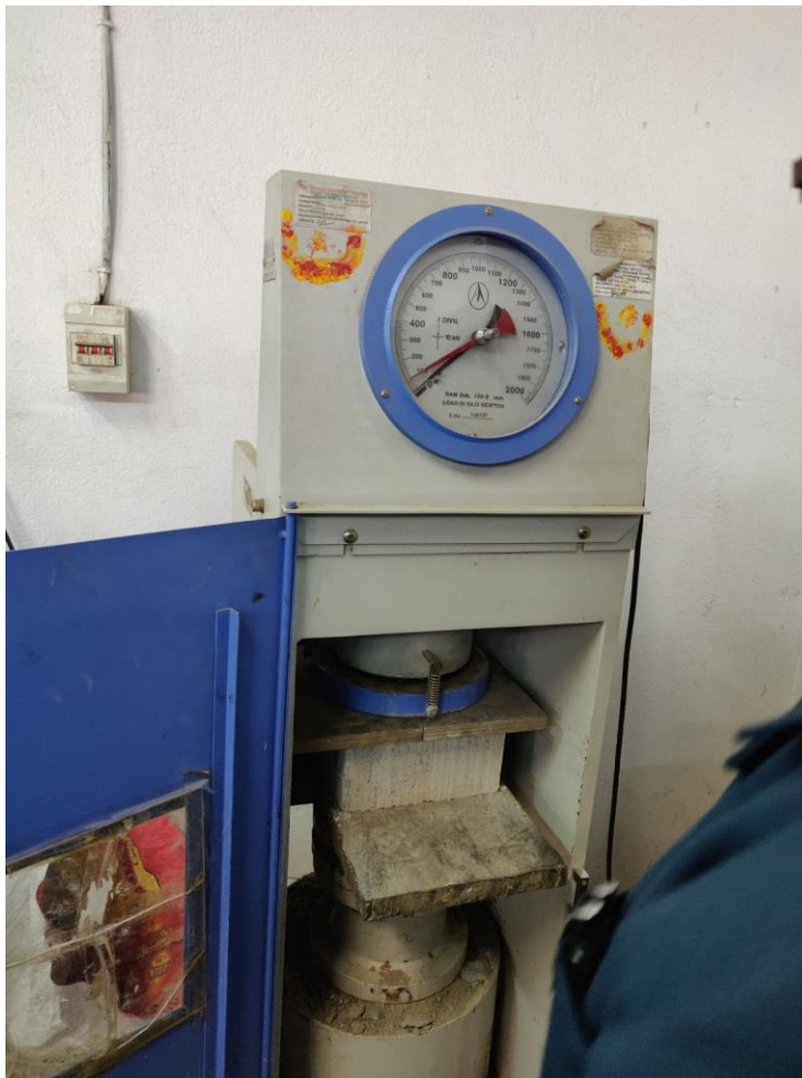
Figure 15 Compression Test of AAC Block
