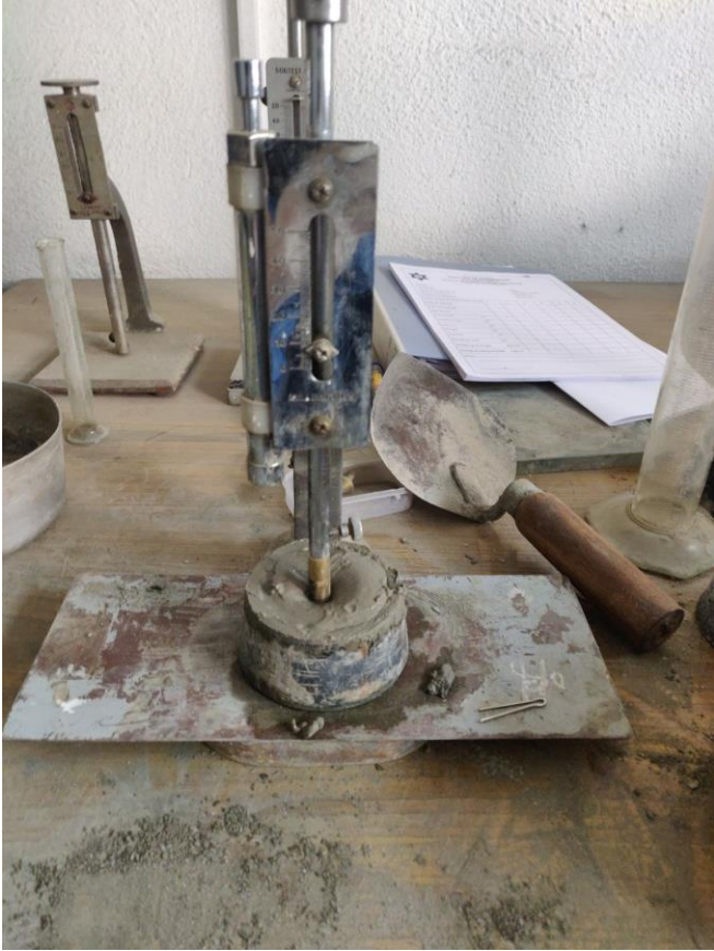
Figure 16 Normal Consistency Test of Cement
