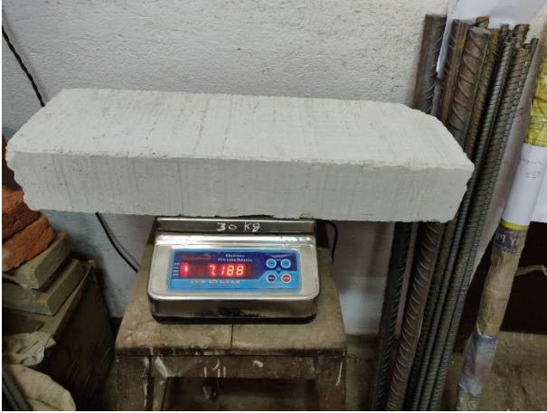
Figure 10 Weighing of AAC before drying
