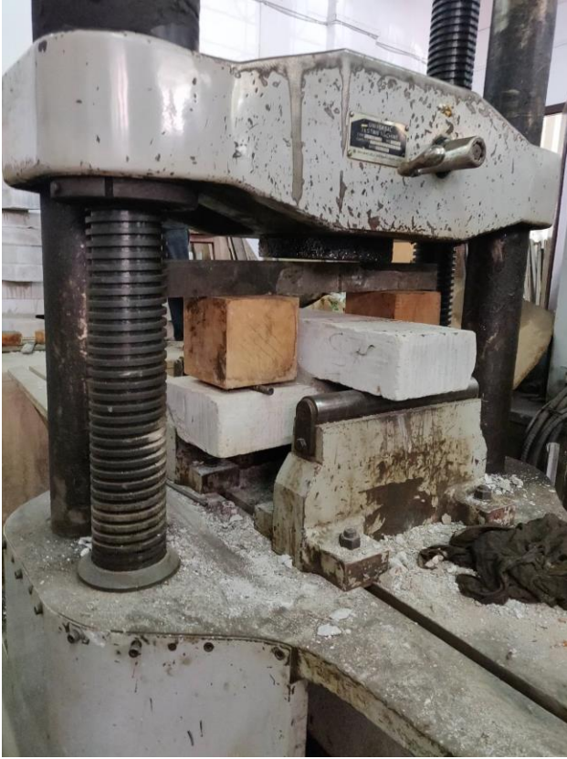
Figure 24 Tensial Strength Test of Cross-couplet Sample
