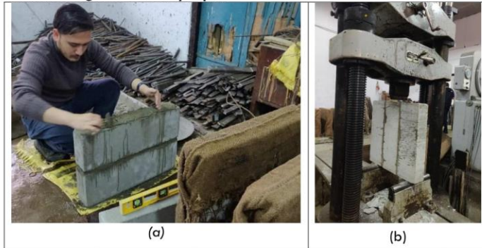
Figure 5 AAC triplet sample: (a) preparation of triplet sample, (b) triplet test
