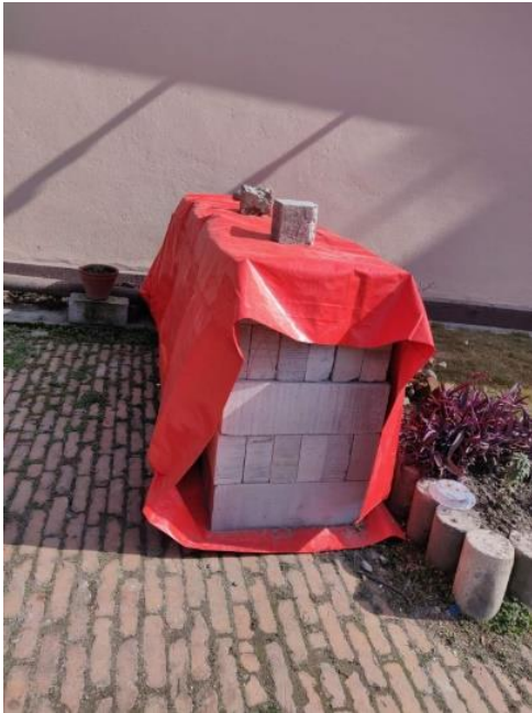
Figure 8 StockPiling of AAC Samples
