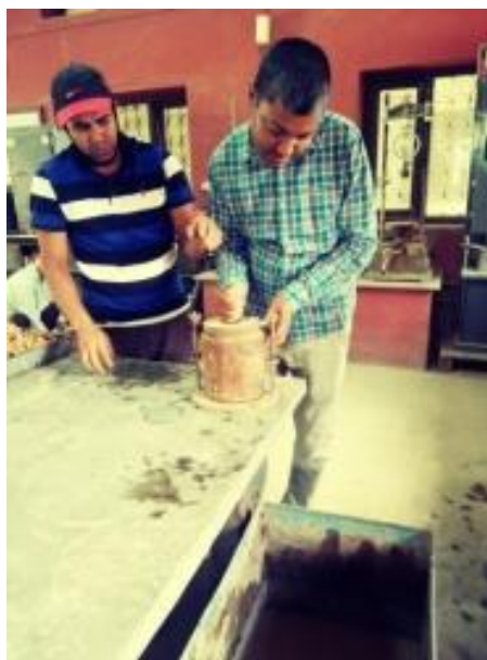
Photograph 0-5 Sample for CBR and Soaking CBR Samples
