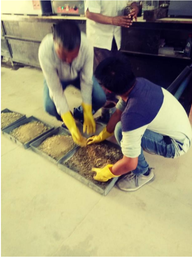
Photograph 0-8 Sample Preparation for Procter Test
