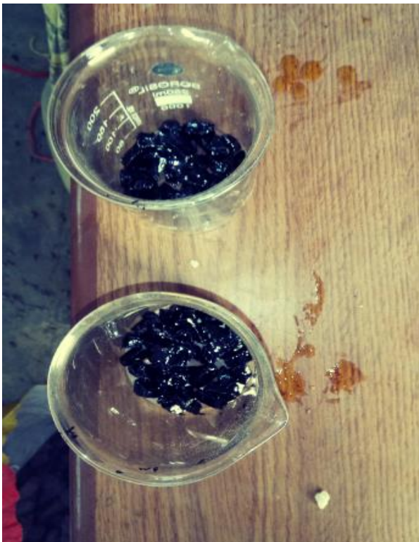
Photograph 0-7 Stripping test sample
