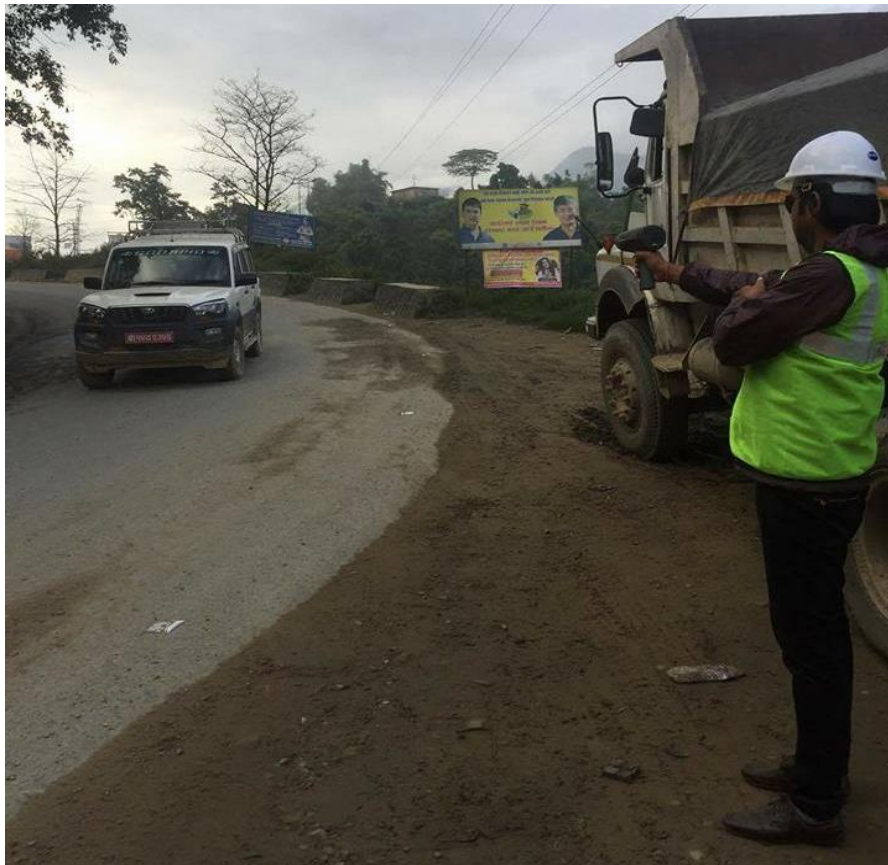
Figure 3.5 Spot speed measurement using radar gun
