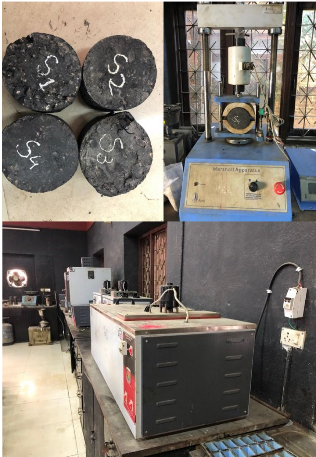
Figure 3. 8 Marshall Equipments for Marshall Immersion test.
