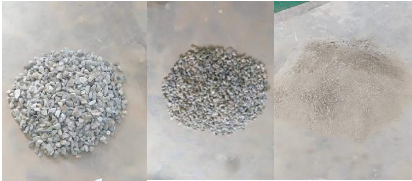
Figure 3. 2 Aggregates used (From the left Agg.-A, Agg.-B, Agg.-C) Gradation curve for the aggregate used is shown in the following figure.
