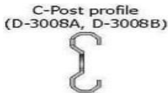
a. Details of cable barrier
