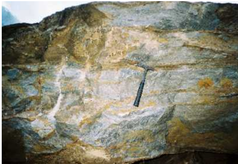
Fig. 4.1 distribution of Phyllite laminations within the Limestone Layer.
