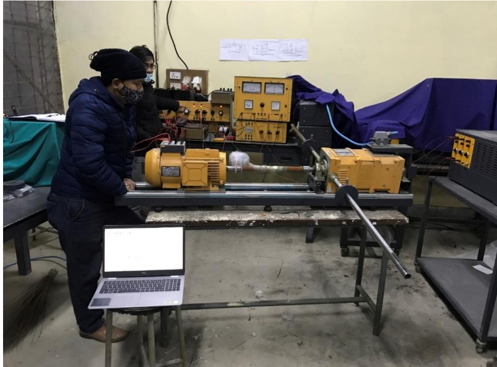
Figure A. 9 Torque transducer calibration
