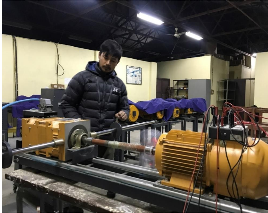
Figure A. 7 Load adjustment during the calibration
