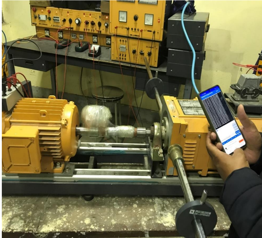
Figure A. 11 Transducer testing and measurement data wireless scrolling on smart phone
