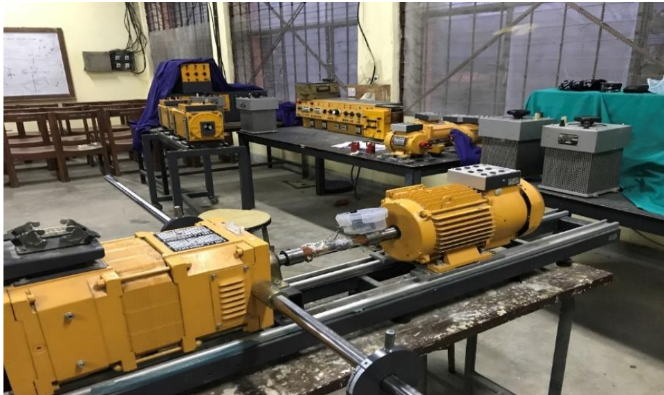
Figure 3. 16 Torque measurement motor generator coupling (DE LORENZO)
