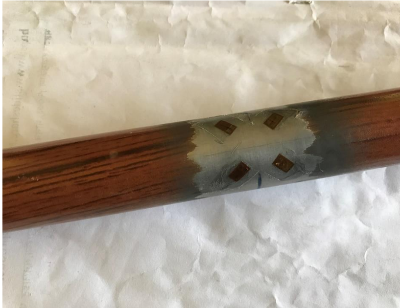
Figure A. 1 Strain gauge glued on shaft at 45^{\circ} to the axis
