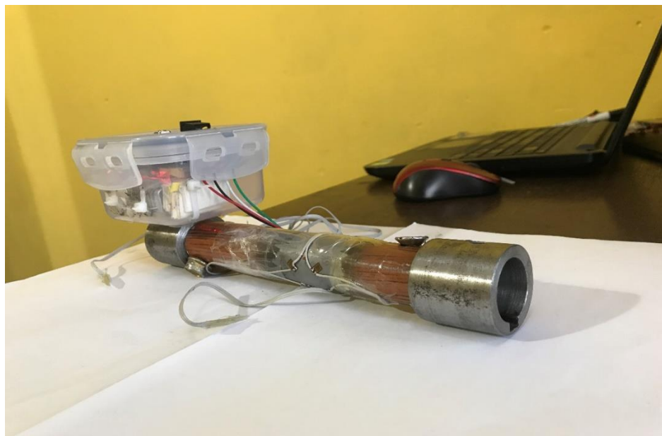
Figure 3. 5 Dynamic torque transducer (constructed in this research)
