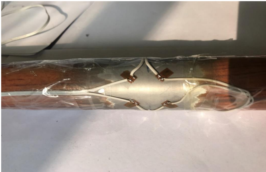
Figure A. 2 Strain gauge wired with Wheatstone bridge pattern
