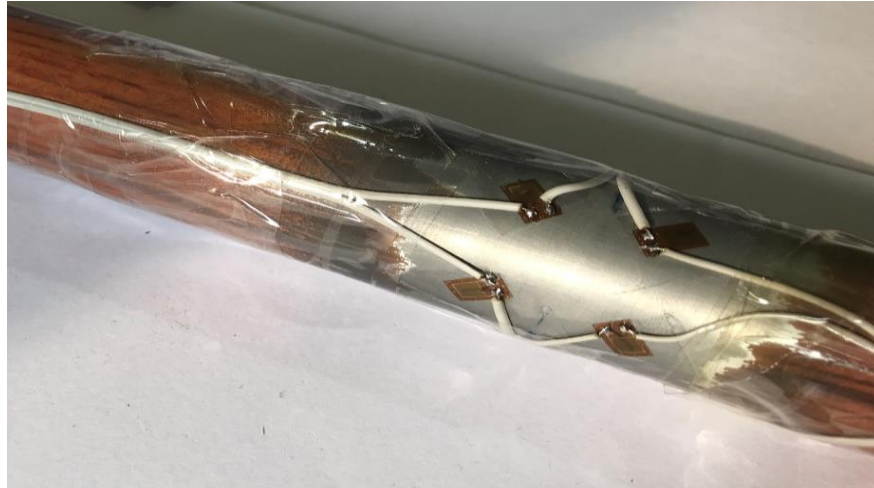
Figure 3. 6 Strain gauges glued on surface of shaft and connection as Wheatstone bridge pattern
