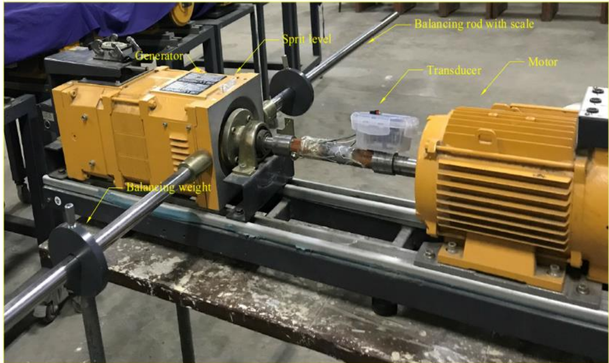
Figure 3. 2 Torque transducer inline couple with generator and motor dynamic torque measurement setup for calibration
