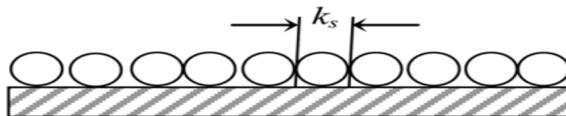
Figure 1.4 Sand-grain height for a uniform sand-grain roughness(Hetsroni et al., 2011)
