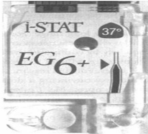
Figure 1.1 Blood Sample cartridge using microfluidic channels(Gad-el-Hak, & Seemann, 2002)
