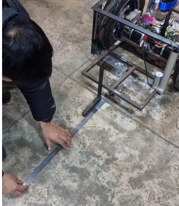
Figure 3.31: Checking the accuracy of odometry
