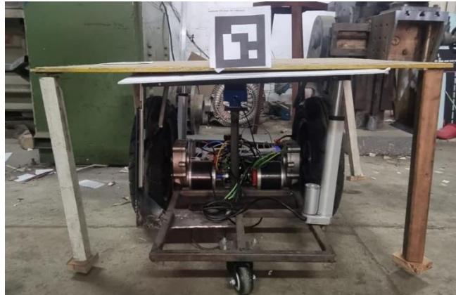
Figure 4.8: Autonomous docking and lifting of payload by the AMR
