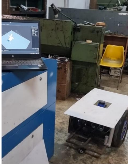
Figure 3.36: Mapping of the real environment using Slam Toolbox
