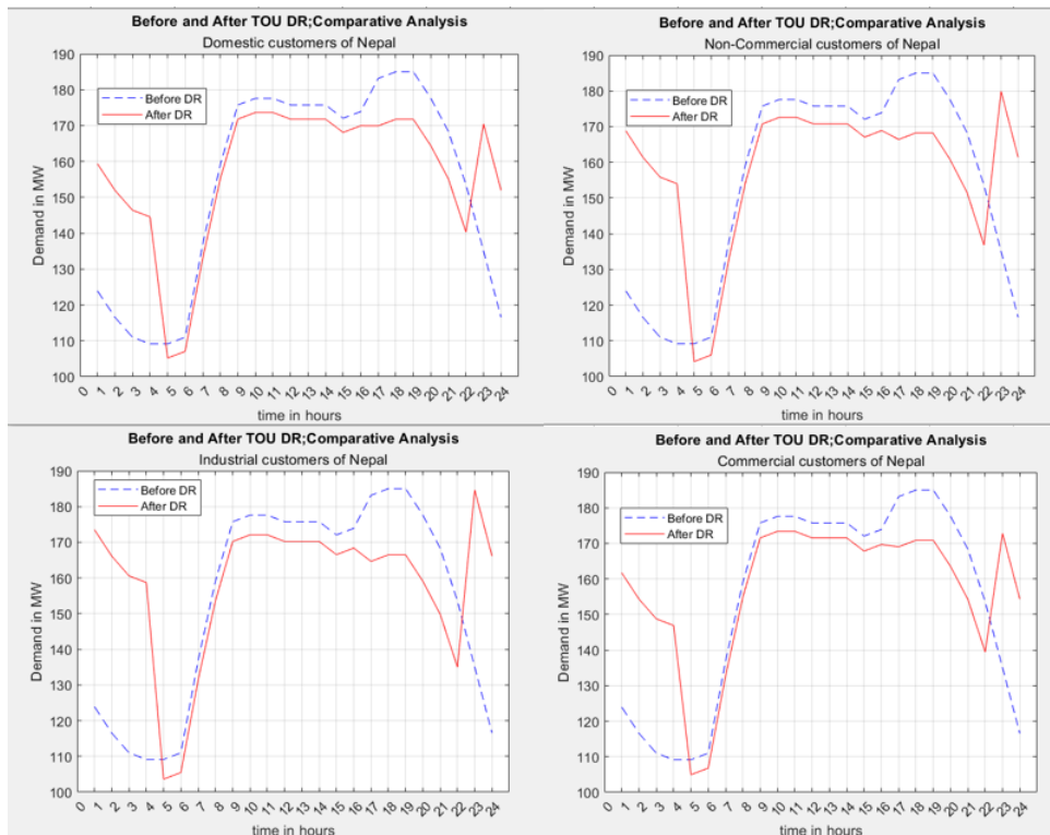
Figure 1. Changes in the peak demand after using TOU DR programs on various type customers of Nepal.
