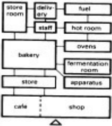
5 Functional diagram for a bakery: good ventilation needed, possibly dehumidify
