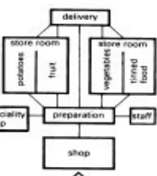
7 Functional diagram for fruit and vegetable shop: little storage provision as most goods delivered daily
