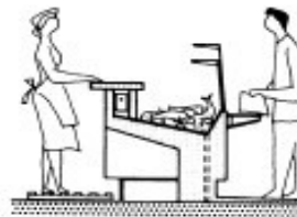
2 Fish counter with cooling compartment and drain
