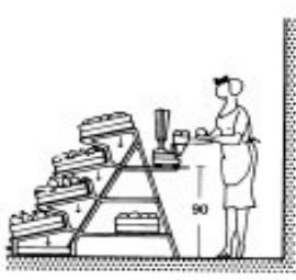
8 Counter with stands for boxes and baskets, drip pan and dirt trap
