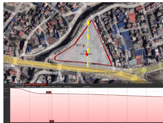
Profile from South to North Level difference 13'-0"
