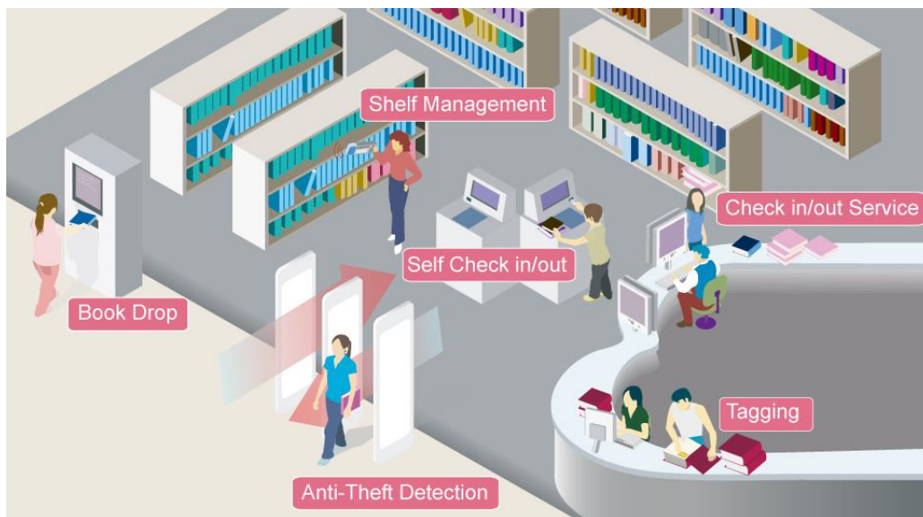
Figure 45: RFID System for library theft detection system
