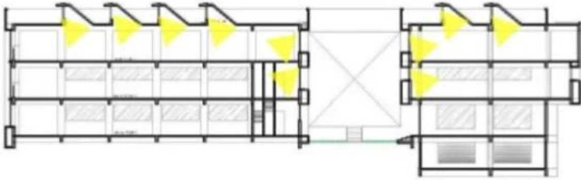
Figure 81: Light through skylight provided on the roof
