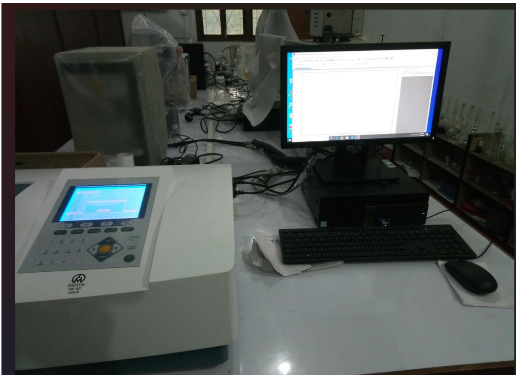
Double beam (MARS ME-SP 195UV, India) spectrophotometer set up with desktop
