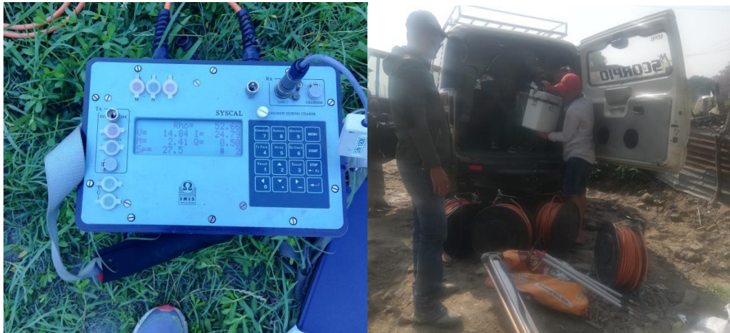
Figure 5: Equipment for ERT survey a) Resistivity meter and b) Necessary accessories
