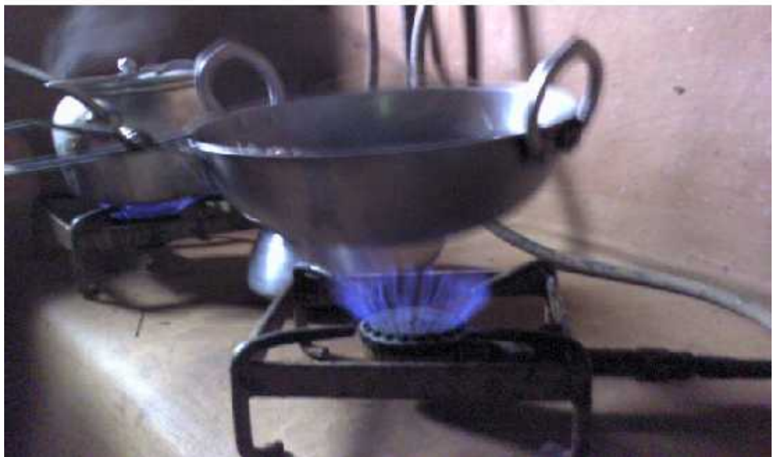
Biogas is burning with blue flame in the double stove
