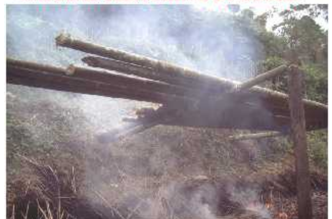
Traditional treatment of Bamboo by smoking
