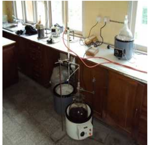
Extraction of oil using Clevenger apparatus
