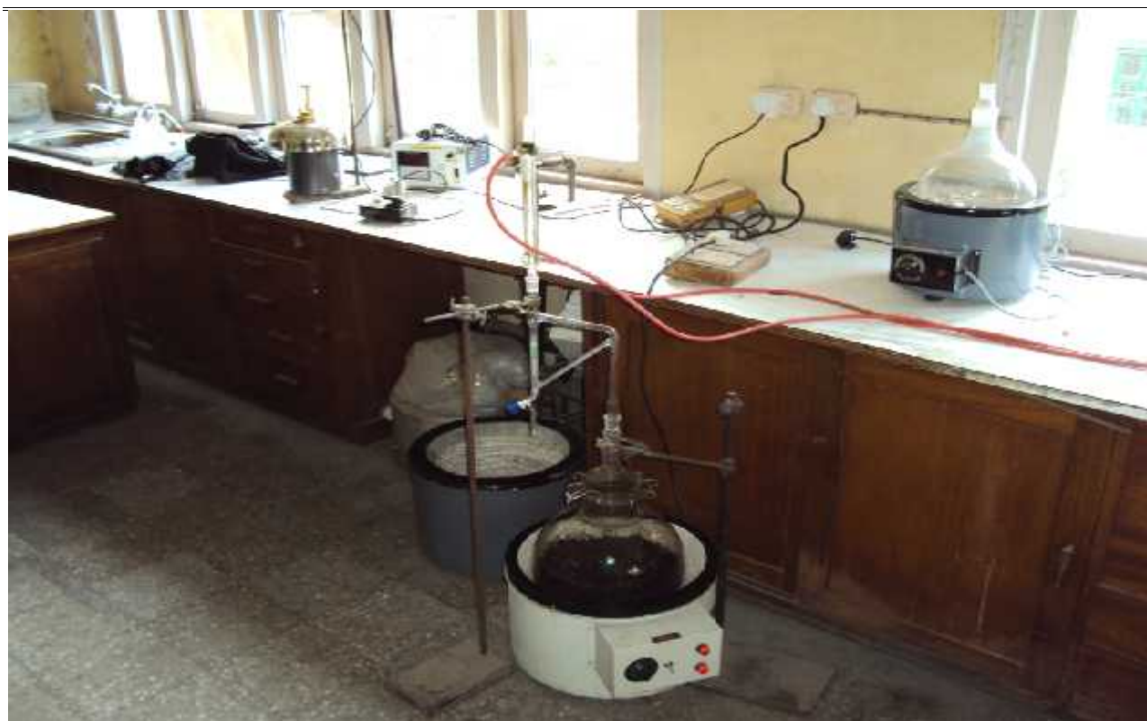
Extraction of oil using Clevenger apparatus
