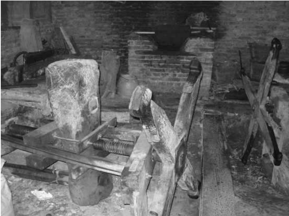
THE TRADITIONAL WAY OF MANUFACTURING MUSTARD OIL
