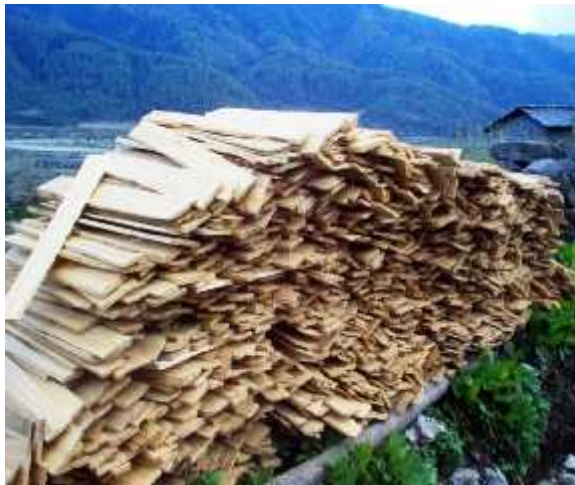
Plate 3: Wooden tiles stacked for roofing houses.
