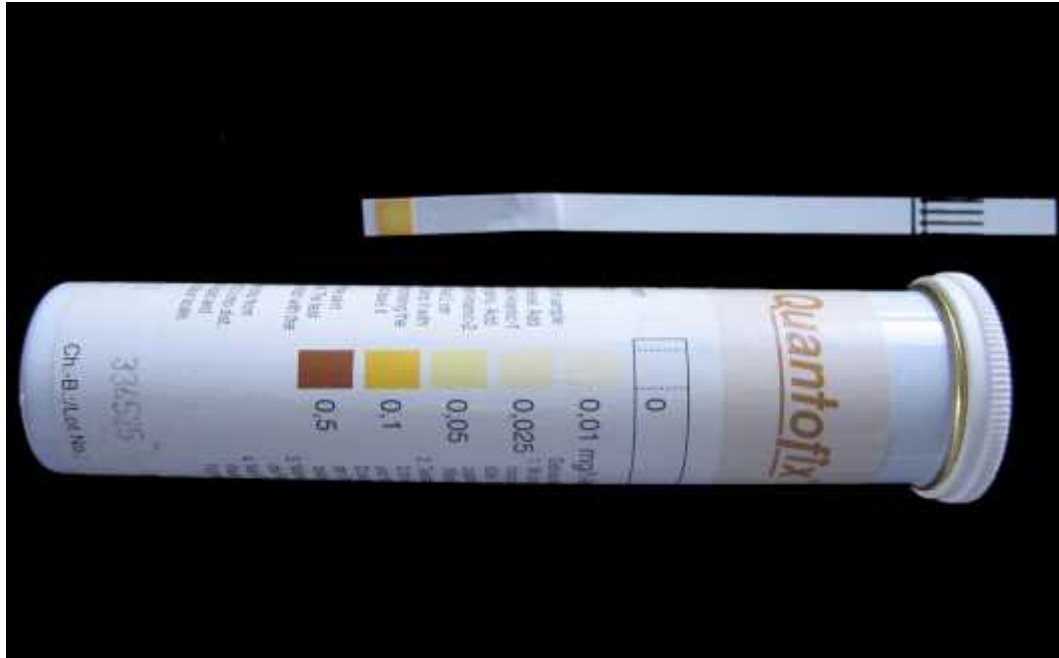
Photograph 3: Arsenic determination by Quantofix test kit
