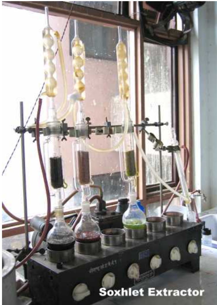
Photograph 2: Soxhlet extractor showing ethanol extraction of medicinal plants
